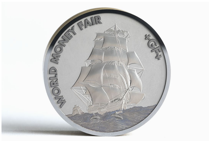
Fig 3: Tungsten carbide HM HS40. Engraving time 9 hours 11 minutes 17 seconds; cleaning and frosting-28 minutes 33 seconds.
