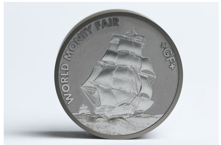
Fig 2: Steel K390 62 Hrc. Engraving time 11 hours 30 minutes 27 seconds; cleaning and frosting 28 minutes 5 seconds; maximum engraving depth 30mm. (image)
