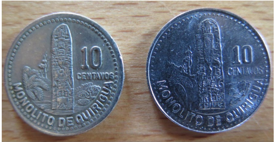
Fig 1: A high quality minted coin (left) and a poor quality minted coin (right) which lacks depth and sharp edges, would not be liked by the public, would not be accepted by vending machines and would soon be rejected in circulation. Its circulation life would be short.
