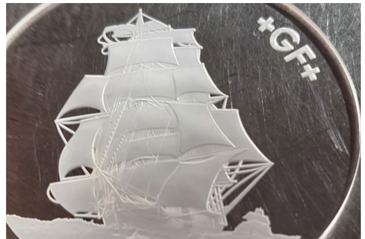
Fig 4: Sapphire. Maximum engraving depth 1.1mm. Engraving times – sea 6 hours 45 minutes, GF logo 16 minutes. There were no cracked edges, no grainy textures, no remelted surfaces and it was reproduced with great detail.
